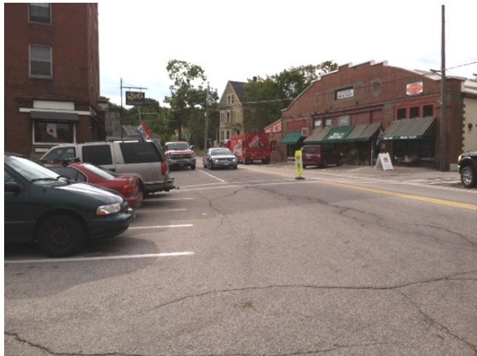
On-street parking restricts sight distance
